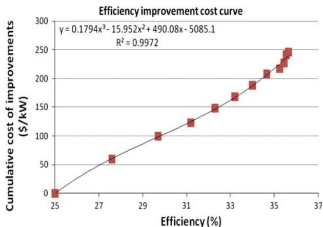
**Fig. 1** Power plant efficiency improvement cost curve. *Source* National Energy Technology Laboratory, “Development of a Cost Curve for Efficiency Improvement Projects at Coal-fired Power Plants,” May 2009
